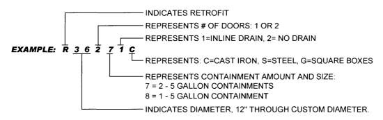
CALL FOR INFORMATION ON RETROFITTING ANY OTHER MANUFACTURER'S BOXES TO SNAP-TIGHT WITHOUT BREAKING OUT CONCRETE!
